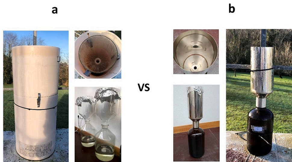
Fig. 1. Photographs of the samplers used in this study: (a) commercial Depobulk®, and (b) EnviroPlaNet sampling device.
